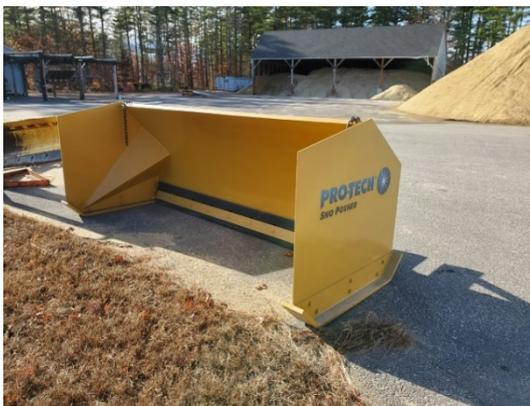
We also fabricated in house, a salt pusher which allows us to stack salt much higher in our shed, effectively increasing our storage capacity, which gives us much needed extra security that we will not run out of salt when the supply chain becomes unreliable as it does after several back-to-back storms when statewide demand is very high.
